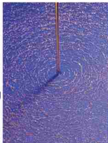
Fig ( 2 – 1) Pattern of iron filings around a wire carrying current
