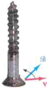
Fig ( 2 - 4 ) Right hand screw direction of screwing.
