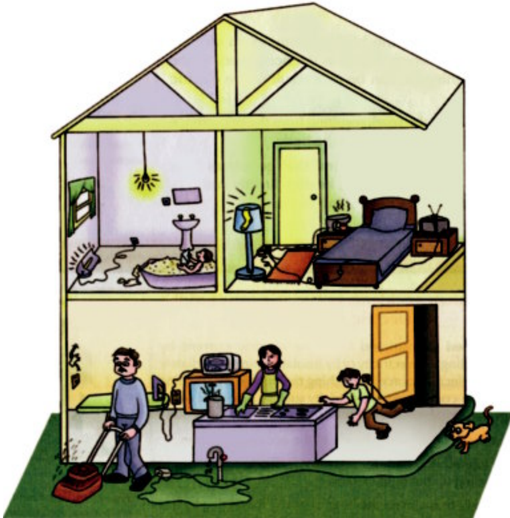
Fig (2-23): Precautions in dealing with electricity:
