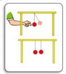
On displacing the pendulum, a work is done, this work is stored in the form of potential energy. When it is left the potential energy is converted gradually into kinetic energy till it reaches a maximum speed where all of its energy is converted into kinetic one.
