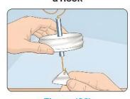
Figure (26) (8) Hang the two foil pieces in the hook and ensure they do not touch each other
