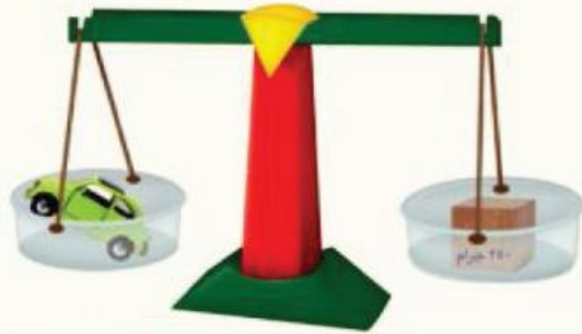
Fig (1-6): Two-arm scale with mass known weights
