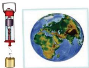
Fig (1-13): The object's weight on the Earth's surface is equal to 6 Newton.
