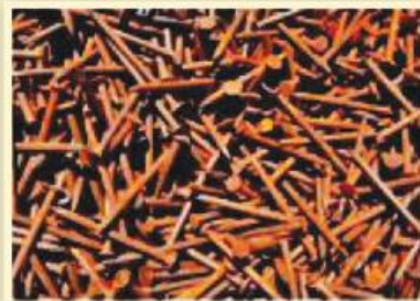
Fig (3-10) Rusty nails after exposure to moisture
