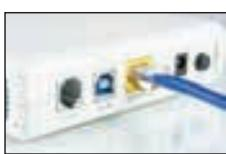
**ethernet port:** connects an ethernet cable; ethernet is more stable and faster than Wi-Fi
