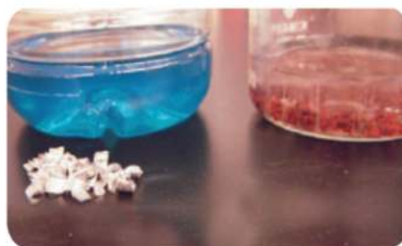
▲ Figure (9) : Substitution of a metal instead of another one in one of its salt
