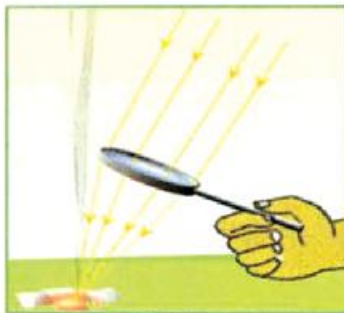
▲ Figure (16): The convex lens forms a real image of the sun on a piece of paper
