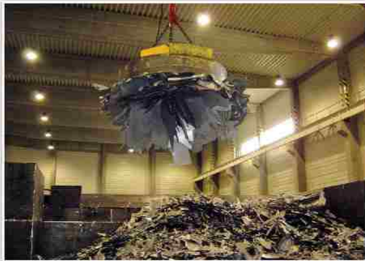
Fig. (24) Electromagnet attracts iron pieces, By turning the electric current off it loses its magnetic force and iron pieces fall.
