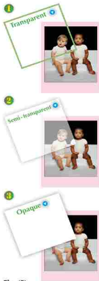
Fig. (5) Light transmission through different materials
