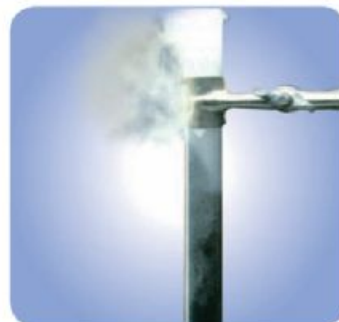
▲ Figure (30) : Manganese dioxide helps in the increase of hydrogen peroxide decomposition speed.
