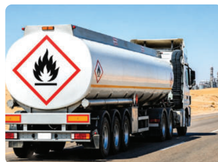
Figure (3) Warning sign for flammable materials
