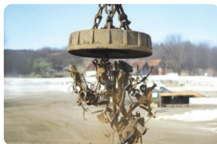
Figure (1) Iron scrap lifting machine
