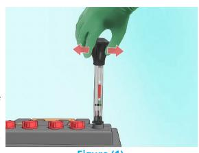
Figure (1) Measuring the Density of the electrolytic Solution in a Car Battery
