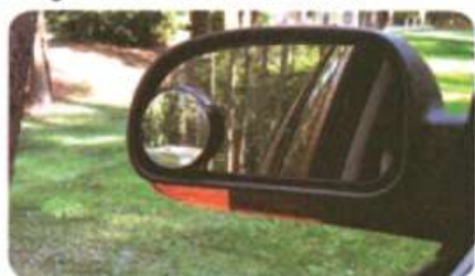
▲ Figure (8): The image that is formed by the convex mirror is virtual, upright and smaller than the object.
