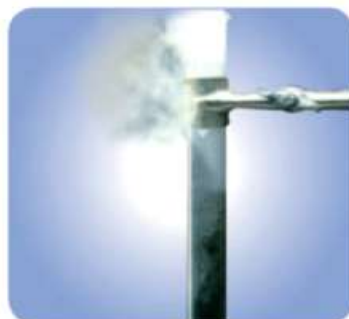
▲ Figure (30) : Manganese dioxide helps in the increase of hydrogen peroxide decomposition speed.
