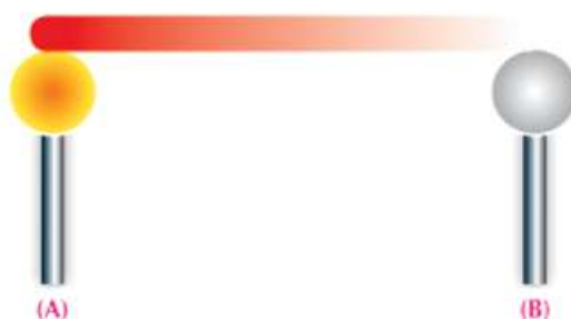
▲ Figure (5) : Heat transference by conduction
