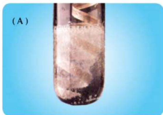
▲ Figure (24) : The reaction of a magnesium ribbon with diluted hydrochloric acid
