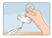
Figure (23) (5) Bend the straight end of the copper wire into a hook
