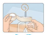
Figure (27) (9) Fix the cap tightly on the glass bottle with duct tape
