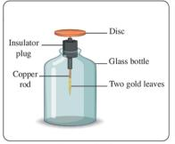
Figure (31) The electroscope
